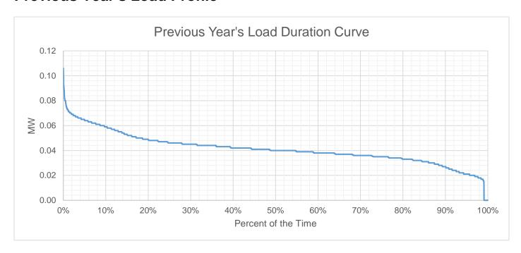
Based on the Load Duration Curve, the minimum load is 0 MW and the maximum load is 0.112 MW for the last historical year.
