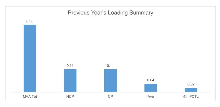
The Non-coincident Peak Demand is 0.11 MW, which is around 34% of the total substation capacity of 0.330 MVA. The load factor or the ratio between the Average Load of 0.04 MW and the Non-coincident Peak Demand is 36% of. A safe estimate of the true minimum load is the fifth percentile load of 0.02 MW which is 18% of the Non-coincident Peak Demand.
