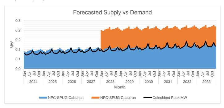
The available supply that ranges from 0.09 MW to 0.13 MW will solely come from NPC's Cabul-an Diesel Power Plant.
