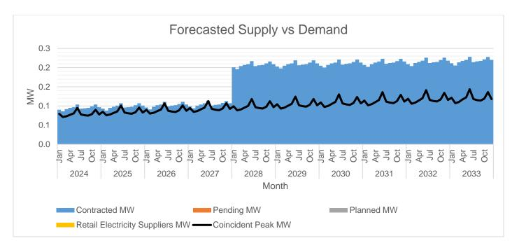
The available supply is generally above the Peak Demand. This is because of the number of diesel generators installed on the island. There are currently six (6) diesel generators on the island with a total plant capacity of 0.474 MW.
